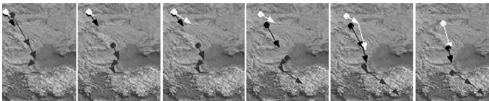
Fig. 5. The time window technique in animation of object movement. The screenshots represent the appearance of a fragment of a map at six consecutive animation moments. The length of the time window is 5 days, that is, each screenshot shows route fragments passed by the moving objects during 5 days. In the second and subsequent screenshots, the time window is shifted by 1 day forward relative to the preceding image. Note that movements of a particular object did not necessarily occur every day.
