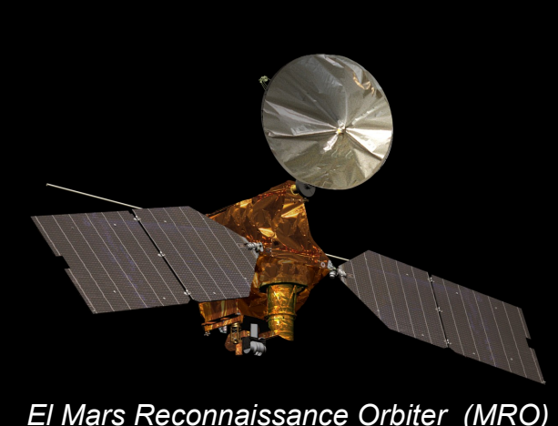
El Mars Reconnaissance Orbiter (MRO) porta el instrumento High-Resolution Imaging Science Experiment (HIRISE).
